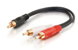
This cost-effective, high quality cable is superior to most standard audio cables, and provides a crisp, clear sound. The dual conductor is 26 AWG 90% spiral-wrapped copper shielded wire to shield against EMI/RFI interference. The connectors are fully molded to provide excellent strain relief while gold terminals ensure long-lasting, corrosion-free connections. Use this cable to split a signal, or adapt from one connection to another.
