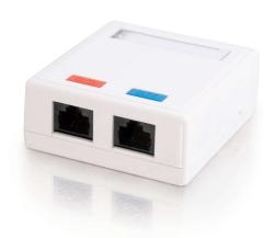
Ideal for surface mount applications, especially in confined spaces. Mount for either side or base entry of cables. Boxes come with mounting screws and adhesive tape, and a cable tie for strain relief. The snap-on cover enables easy closure or access for quick installation. Each box includes a write-on label with holder for easy designation of different system or station. Contacts are phosphor bronze plated with 50 inch hard gold.
