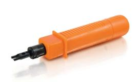
This impact punchdown tool has an impact mechanism inside divided from the turnable body. It also has a rugged frame with a storage compartment in the tool's body for storing one blade. Made from hardened SNCM-21, the blade is interchangeable and reversible - very convenient. Plus, you can quickly change the blade without using a screwdriver.
