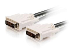
This precision-engineered cable is fully compliant with the DVI standard defined by DDWG (Digital Display Working Group). The DVI-D dual link configuration provides enough bandwidth for resolutions up to 2560x1600 pixels and allows high speed digital video transmission up to 9.9 Gbps. 28 AWG copper conductors are individually insulated in foam-polypropylene to minimize crosstalk, and ensure high speed, error-free transmission.
