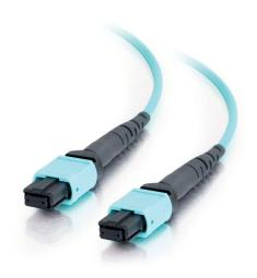
Make MTP/MPO your choice for high density fiber networks; it's specifically designed for fast ethernet, fiber channel, ATM and gigabit ethernet applications. Save time and money with MTP/MPO's increased ease of installation - simply pull one cable rather than twelve. Each MTP/MPO fiber assembly consists of twelve laser-optimized, 10G 50/125 multimode fibers under one OFNP plenum-rated jacket.
