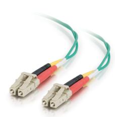
With LC to LC termination, this high quality fiber optic patch cable is specificially designed for ethernet, multimedia, or communication applications. The small LC connector [B]takes HALF the size of traditional SC and ST fiber connectors,[/B] since it offers twice the port density of conventional SC and ST connectors to satisfy the need for higher port density in telecom closets, equipment rooms, and work areas.
