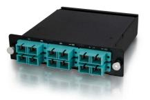
Small form factor: 1.125in x 5.125in x 4.5in. This breakout module provides the mechanical distribution of the 12-strand MTP/MPO connector. Housed in a rugged steel enclosure guaranteed for life, this durable module arrives fully loaded with the preterminated and tested MTP/MPO breakout harness. It is shipped with a test report that can assist in calculating the optical budget.
