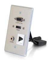
The HDMI, VGA, 3.5mm and Keystone Pass-through Wall Plate is perfect for the transition to in-wall cabling. The HDMI pass-through port includes a thin, flexible HDMI pigtail that accommodates the tight bend radius required for installations within a standard junction box. The keystone allows for integration with new or existing cable infrastructure for telephone or Ethernet. Constructed of aircraft grade aluminum, this wall plate is designed for durability and a long life.
