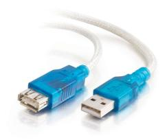
This extension cable actively buffers the incoming and outgoing signals to ensure compliance with the USB 2.0 specification for electrical and timing minimums. You can connect up to 3 active extension cables end-to-end to achieve up to 118 feet (36 meter) total extension! Both low and high speed USB devices will function equally well with this extension cable. The active chip is built into the female connector so you can easily install this cable in conduit or raceway!
