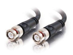
A high quality BNC cable for video applications including CCTV, broadcast, studio, boardroom presentations, home theater, etc. Manufactured from 75 Ohm RG59/U dual shield coax cable (60% copper braid over foil) with a 22 AWG copper-covered steel center conductor. Finished with bright nickel-plated BNC connectors that have molded PVC strain relief to protect the cable from wear over time.
