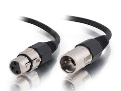
Use this XLR to XLR cable to connect unbalanced sources to balanced XLR inputs. This pro-audio cable is made from 22 AWG twisted pair audio cable under an aluminum foil shield and 60% copper braid for maximum shielding from noise. The highly flexible 7mm PVC jacket reduces the risk of the cable kinking and damaging the conductors.
