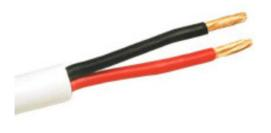
This is the right cable to install audio throughout your house. Made from 65 strands of 99.9% high-purity copper, this speaker wire is very flexible and less likely to kink during installation. CL2-rated for use inside walls, this wire features a flame-retardant white PVC jacket that helps to diminish the potential of fire spreading between floors.
