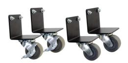
The Caster Kit is designed exclusively for the Legrand® Swing-Out Wall-Mount Cabinets and is a perfect solution for maneuvering cabinets in floor applications . Do not worry about free motion or uncontrolled rotating, as the kit includes 2 swivel non-locking casters and 2 swivel locking casters which offers steering in a controlled direction. The caster mounting features a load rating up to 300 lbs plus the weight of the unit, with each caster rated at 150 lbs.
